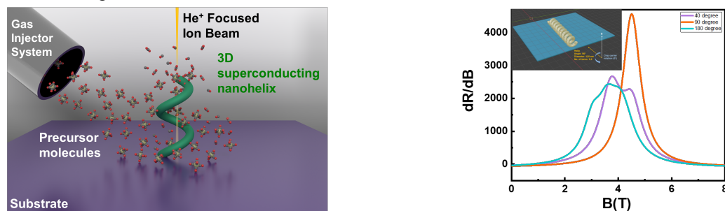
Figure 1. Left: Schematic of direct-write growth of a 3D W-C nanohelix by He + -FIBID. Right: Representative angle-dependent R(B) curves of a nanohelix. The inset shows a sketch of the measured nanohelix geometry and mounting orientation.
